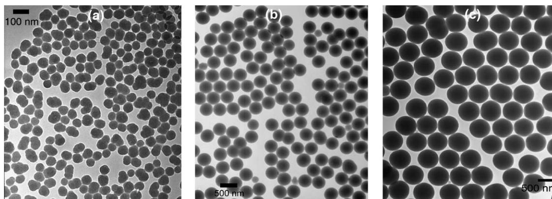
Fig. 1. Transmission electron microscopy (TEM) images of Ru(phen)<sub>3</sub> containing silica particles prepared using the Stöber method. In image (a) the scale bar is 100 nm. In images (b) and (c) the scale bar is 500 nm.
