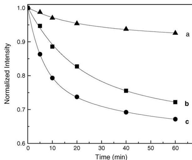
Fig. 2. Photostability measurements: (a) fluorescent silica particles prepared using the one-pot Stöber method, (b) fluorescent silica particles prepared by loading Ru(phen)<sub>3</sub> into pre-prepared silica particles, and (c) a solution of 0.1 mM Ru(phen)<sub>3</sub>. The samples were excited with a 1.5 KW Xenon lamp in a Suntest CPS+ Instrument.
