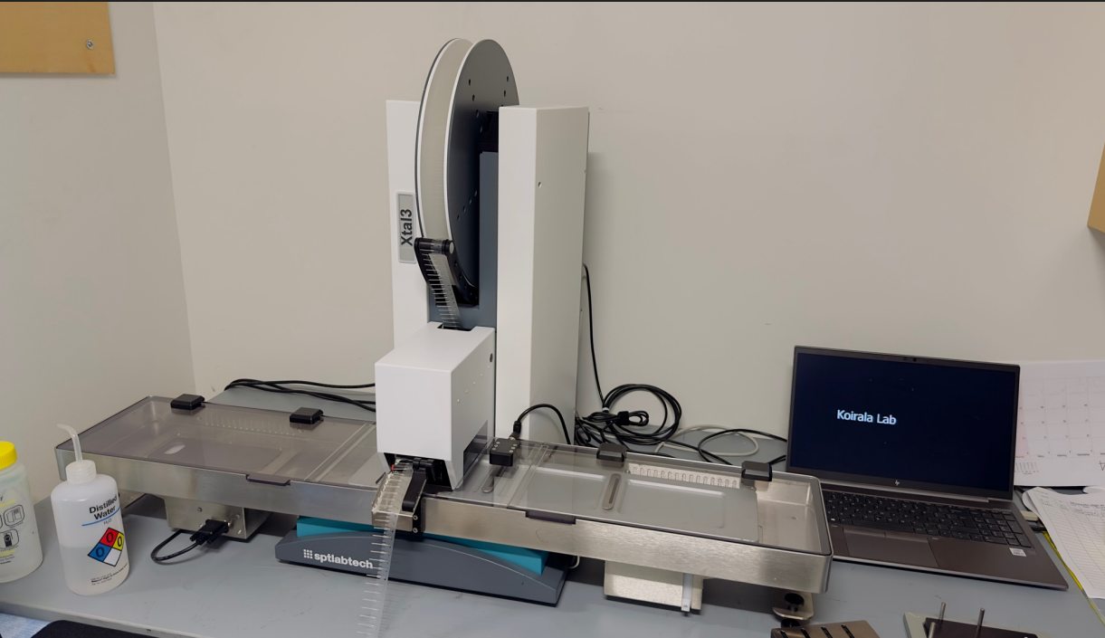
Crystallization Robot Mosquito Xtal3
